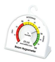
The general purpose hygrometer incorporates a 70 mm diameter dial with arrow indicator and colour-coded zones to display humidity levels e.g. dry, moderate and humid. The hygrometer indicates the level of humidity in 5 % divisions over the range of 0 to 90 %rh.
